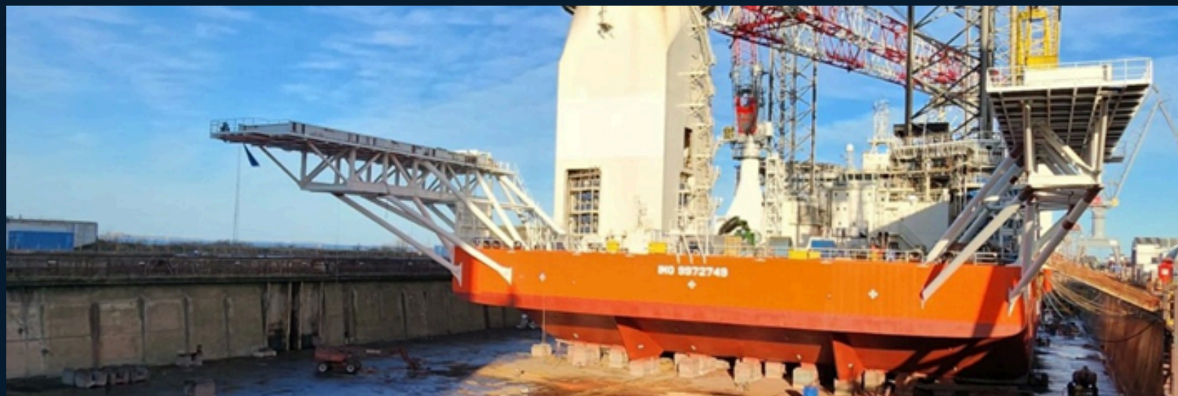
Dry Dock 2200mt (LEC) Leg Encircling Crane
